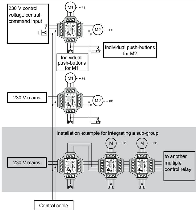
**i** An additional multiple control relay is needed for each sub-group. In this installation example, one drive is controlled in the sub-group per multiple control relay. Alternatively, 2 drives can also be operated on one multiple control relay, as shown above.
